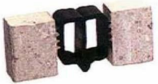
Figure 1: Masterflex J Seal neoprene profile J Seals with 100% movement capability are used for dynamic movement, for example for bridges, viaducts, tunnels, car park structures and water management applications.
